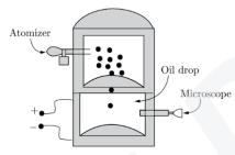
That is, when suspended, upward force qE just equalled Mg. Millikan accurately measured the charges on many oil drops and found the values to be whole number multiples of  $1.6x10^{-19}$ C the charge of the electron. For this, he won the Nobel prize.
