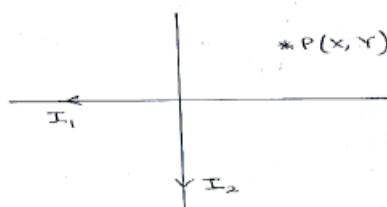
Magnetic field due to conductor carrying current  $I_1$   $(\vec{B}_1) = \frac{\mu_0 I_1}{2\pi Y} (-\hat{k})$
